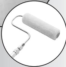
The Inner Feed Pressure Roller is specifically designed for the professional concerned with high production paint applications. The paint distributor mechanism is actually an auger which rotates through the length of the head assembly to evenly distribute paint to all points of the roller cover. It is this device that allows the operator to spend more time applying paint without concern for heavy build-ups or uneven paint distribution.
