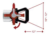
Wide Spray - wide angle / large orifice opening. Ideal for large areas and a high working speed.
